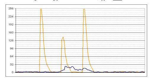
Since the units are only 50m apart the beam divergence is minimal so parallel walking is only detected when very close to the centreline, within 0.5m in this case. Movement beyond 1m from centreline was too low to measure.
