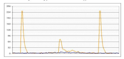
Human walking 2m away from the beam centreline produces a low movement level. Setting a threshold of 32 would easily detect the wanted beam crossing and reject the parallel movement in this situation
