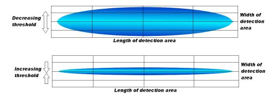
The most accurate method to determine the threshold is to walk parallel to the beam and then cross the beam in a few different locations.
