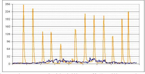
In this case setting a movement level threshold between 32-64 would be appropriate to detect the crossing target but ignore parallel targets 2m away.
