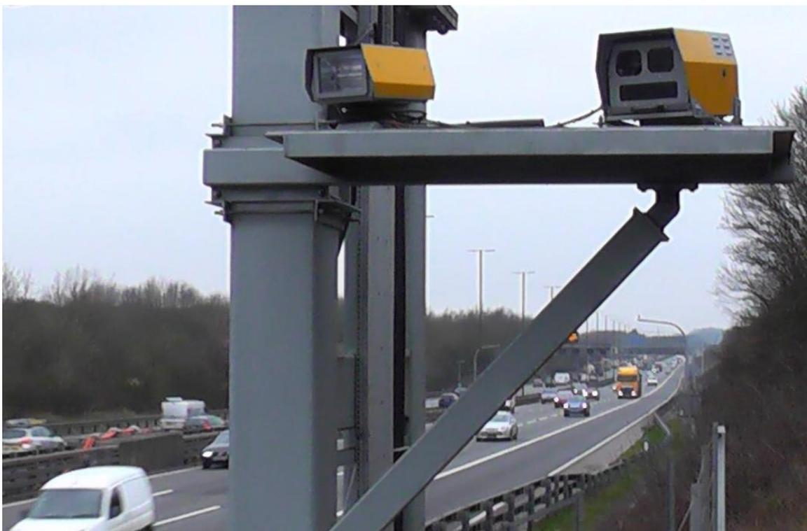
Figure 1 - Typical HADECS3 roadside installation – radar is positioned on the right.
