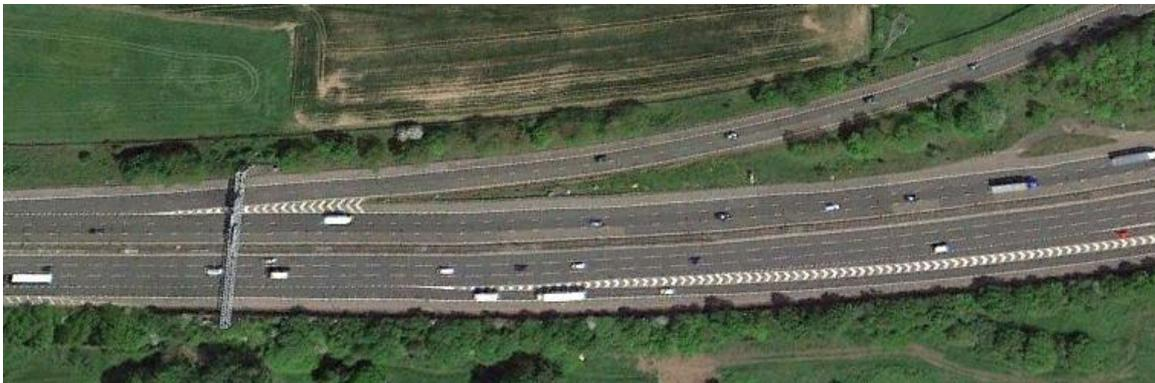
A number of large trees were next to the hard shoulder and allowed us to evaluate how the system would work when vehicles stopped next to the trees. A large gantry was situated around 130m from the radar and allowed us to evaluate the radar's ability to ignore very large static objects in the environment.
