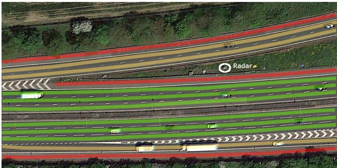
The radar was positioned so that a large number of lanes would be monitored at once. This presented the radar with a very high number of vehicles within the field of view to make the detection algorithms work hard to highlight if there were any flaws in our approach. There were three hard shoulders (red), three slip roads (yellow) and six running lanes (green), giving a total coverage of 12 traffic lanes for a single radar sensor.
