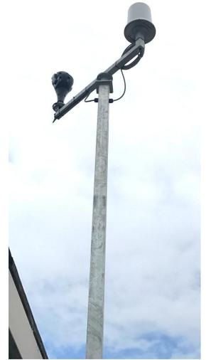
Scan-360 is the ideal solution for securing large areas and compounds. The radar can be mounted high to see over obstructions and does not have a large blind spot underneath. The web-browser based configuration uses an intuitive satellite map, over which the detection areas are defined by simply drawing the required area outlines.
