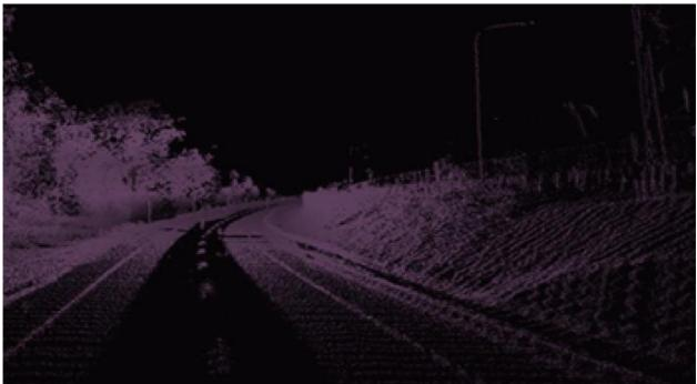
The image above shows typical road scene mapped by a lidar sensor during clear weather. Pixel brightness corresponds to the reflectivity of the surface.
